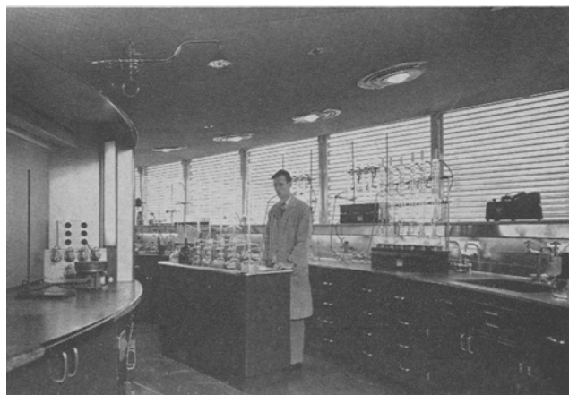
FIG. 2. This is a view of a mezzanine floor, showing fume hood and safety shower.
